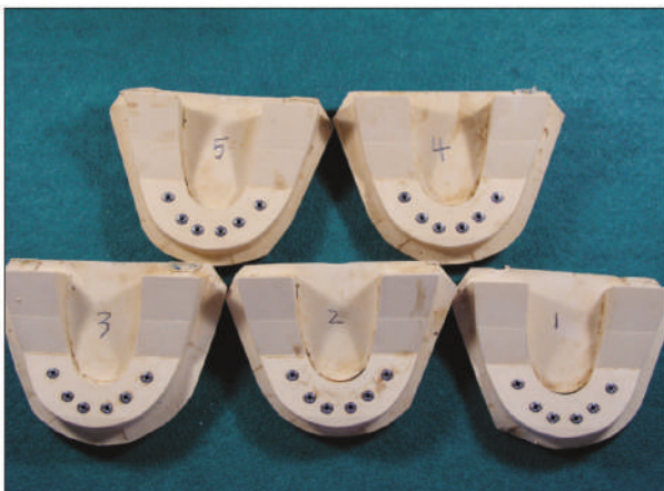
Fig. 10. From master model, 5 impressions and experimental models were made for each splinting method.
